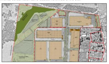
Figure 1: A Master plan showing the flood storage basins
